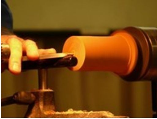
Start hole for screw to fit in for top
