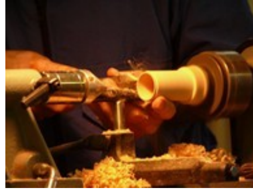
Support when using parting tool
